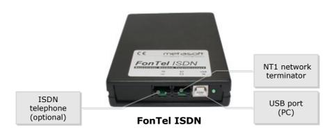
**FonTel ISDN** recorder is connected to the network terminator NT1 (S0 interface) similarly to an ISDN telephone. NT1 network terminator has at least 2 outputs for connecting, for example, two ISDN telephones. If any of the sockets is available, the recorder's **NT** input can be connected to it. If all of the sockets are in use, one of the connected devices shall be plugged out, the recorder (**NT**) is placed instead, and the plugged-out device is connected to the recorder's **TE** socket.
